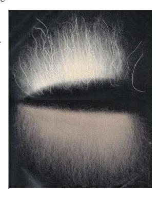
by their high value and ability to be repeatedly processed. This is the reason why, since the end of the 19th century, an organized system of collecting and recycling wool waste through mechanical processing was established. After the mechanical processing of reverse splitting and carding the wool fibres, a reduction in their initial staple length is observed.
