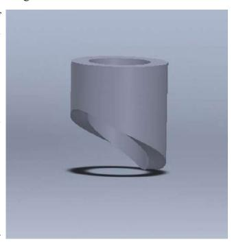
axial movement of the needle. The bearing between the cam and the needle guide is carried out by friction. Insufficient smoothness of the two surfaces will cause additional friction forces. A reduced contact surface will cause abrasion of the two surfaces, more on the less resistant one.
