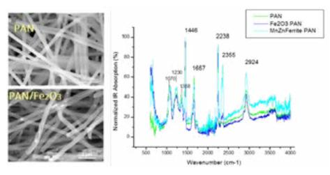
tive clothing, energy storage, catalysts, electric double-layer capacitors. In this study, production and advanced experimental characterizations and interfacial interaction of confined and homogenously dispersed magnetic nanoparticles of iron oxide (Fe2O3) and mangan zinc ferrite (MnZnFerrite) in polyacrylonitrile (PAN) matrix as in the nanofiber form are studied in detail [4].
