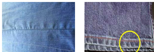
Figure 2. Defects caused by mutual displacement of fabric layers
