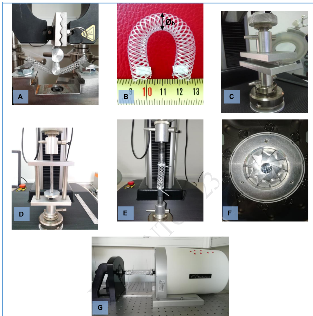
Fig. 3. Characterization methods: (A) Three points bending test (B) Unchanged bending diameter measurement (C) Parallel plates compression test (D) longitudinal compression test (E) Elongation test (F) radial compression test (G) Accelerated fatigue test.
