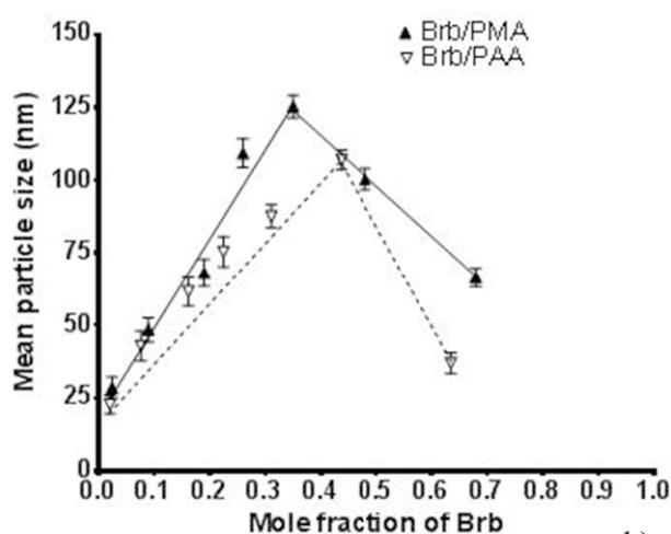
**Figure 5** TEM micrographs of Brb/PMA NPs (mole fraction of Brb of 0.35) (a). Dependence of the mean size (b) on the mole fraction of Brb for Brb/PMA and Brb/PAA NPs at partner concentration of 0.01 wt %; pH 4.9;  $I = 0.1$ ,  $25 \pm 0.1^\circ\text{C}$ .
