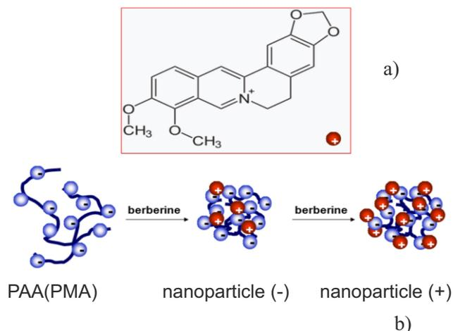
**Figure 4** (a) Structure of Brb, (b) Schematic representation of the preparation of NPs based on complex between Brb and PAA or PMA at pH 4.9.
