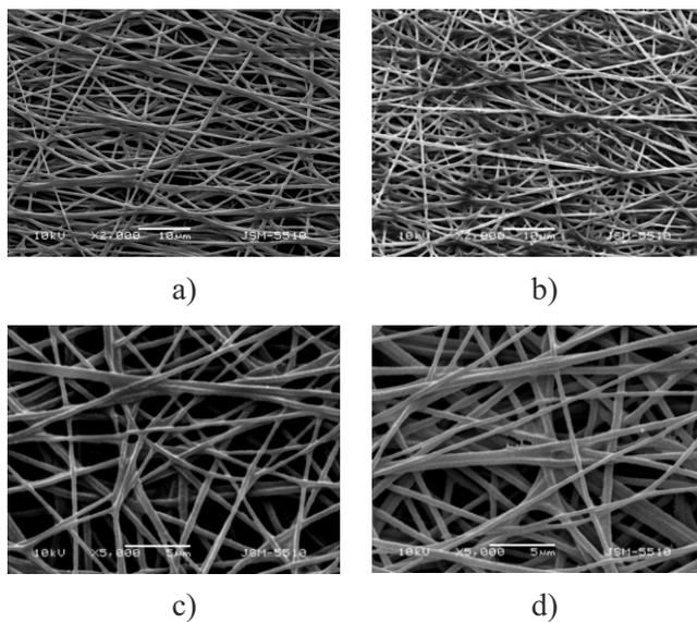
**Figure 2** SEM micrographs of electrospun mats of: Jeff-8Q/inPLA (a), Jeff-8Q.Cu<sup>2+</sup>/inPLA (b), Jeff-8Q/onPLA (c) and Jeff-8Q.Cu<sup>2+</sup>/onPLA (d). Magnification ×2000 (a and b) and ×5000 (c and d).
