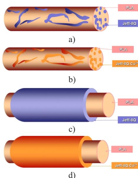
**Figure 1** Schematic representation of fibrous materials type “*in*” prepared by one-pot electrospinning (a,b) and type “*on*” prepared by electrospinning in conjunction with dip-coating (c,d)
