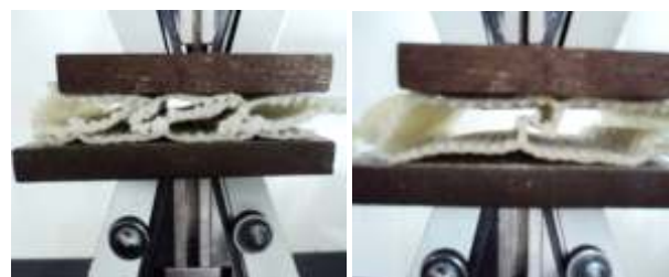
Figure 6 Deformed 3D composites under flat compressive loads: (a) V and (b) U-shaped composites
