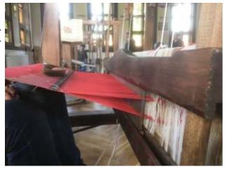
therefore, after each beaten weft the tension in the main threads increases. This changes the conditions of intercrossing and mutual working of the warp and weft threads. From this point of view, hand weaving is not limited by the thread-binding technique but requires additional knowledge and skills on textile materials.
