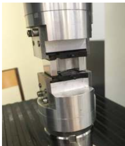
Figure 1 Specific attachments for the MTS device and the Pressley jaws; bundle tests.
